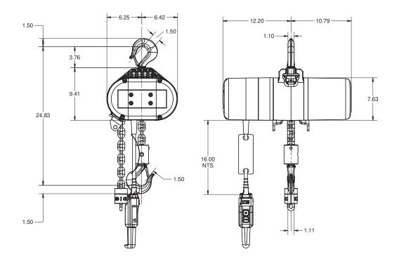
Dimensions (in inches) are RRS model CM Lodestar 2 Ton Single Reeved with Swivel Latch Type Hook Suspension.
