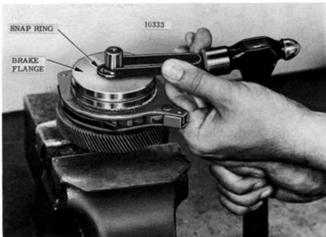
Figure 7-18. Removing Snap Ring from Load Brake Shaft.
