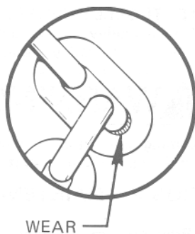
Figure 5-1. Check Chain Wear at Bearing Surfaces Between Links.
