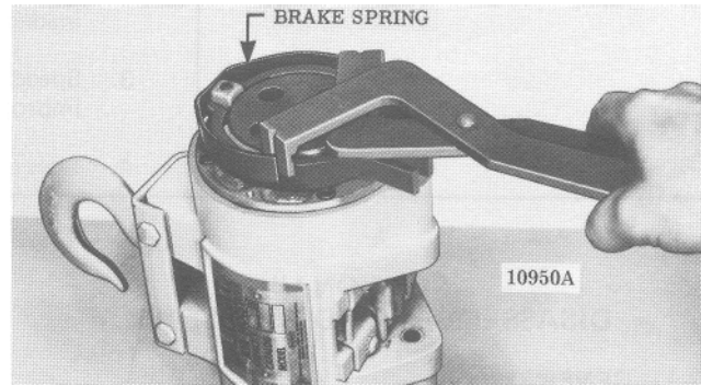
Figure 7-5. Removing Brake Spring Using Special Tool.
