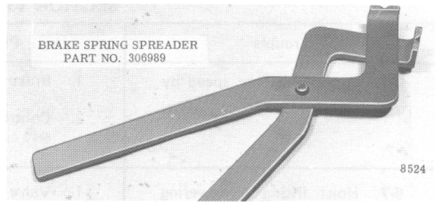
Figure 7-4. Special Tool for Removing Brake Spring.
